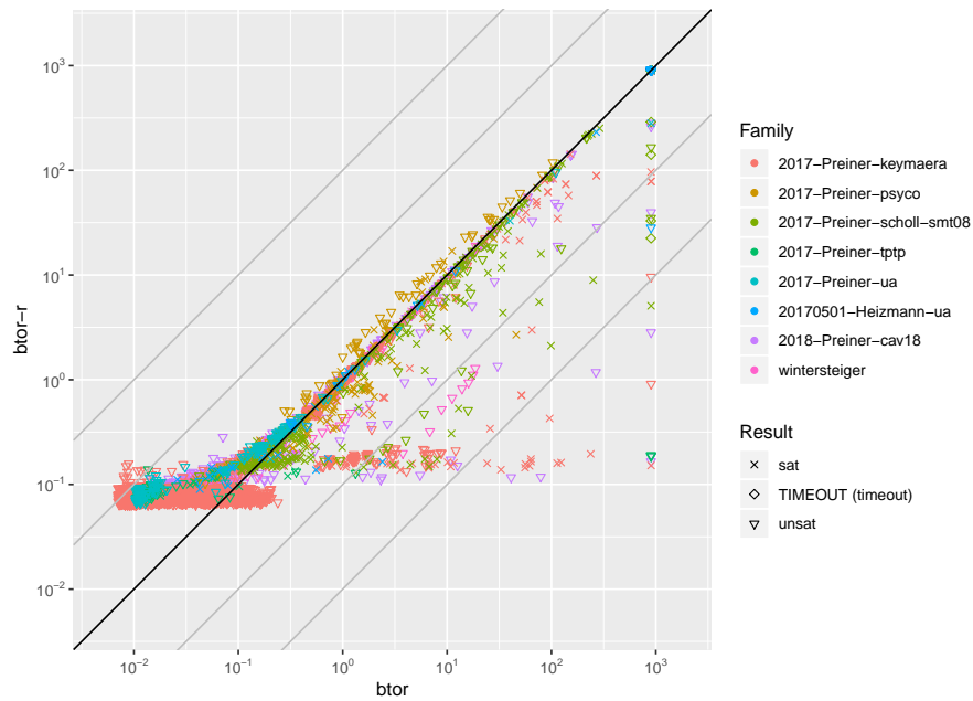
Figure 11.2: Scatter plot of wall times of the solver btor and the solver btor-r. Each point represents one benchmark, its color shows the benchmark family, and its shape shows its satisfiability. The gray lines represent hundredfold and thousandfold difference.
